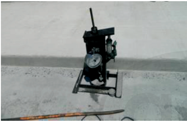
Fig. 5.4a—Tensile bond test apparatus for 2 in. (50 mm) diameter bond tests.
