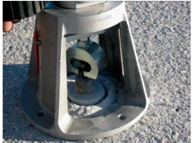
Fig. 5.4b—Tensile bond test apparatus for 1 and 2 in. (25 and 50 mm) diameter bond tests.
